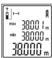
The device will emit an acoustic signal throughout the duration of continuous measurement.
